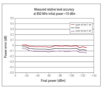
Relative level accuracy measures the accuracy of a step change from any power level to any other power level. This is useful for large changes (such as 5 dB steps).
